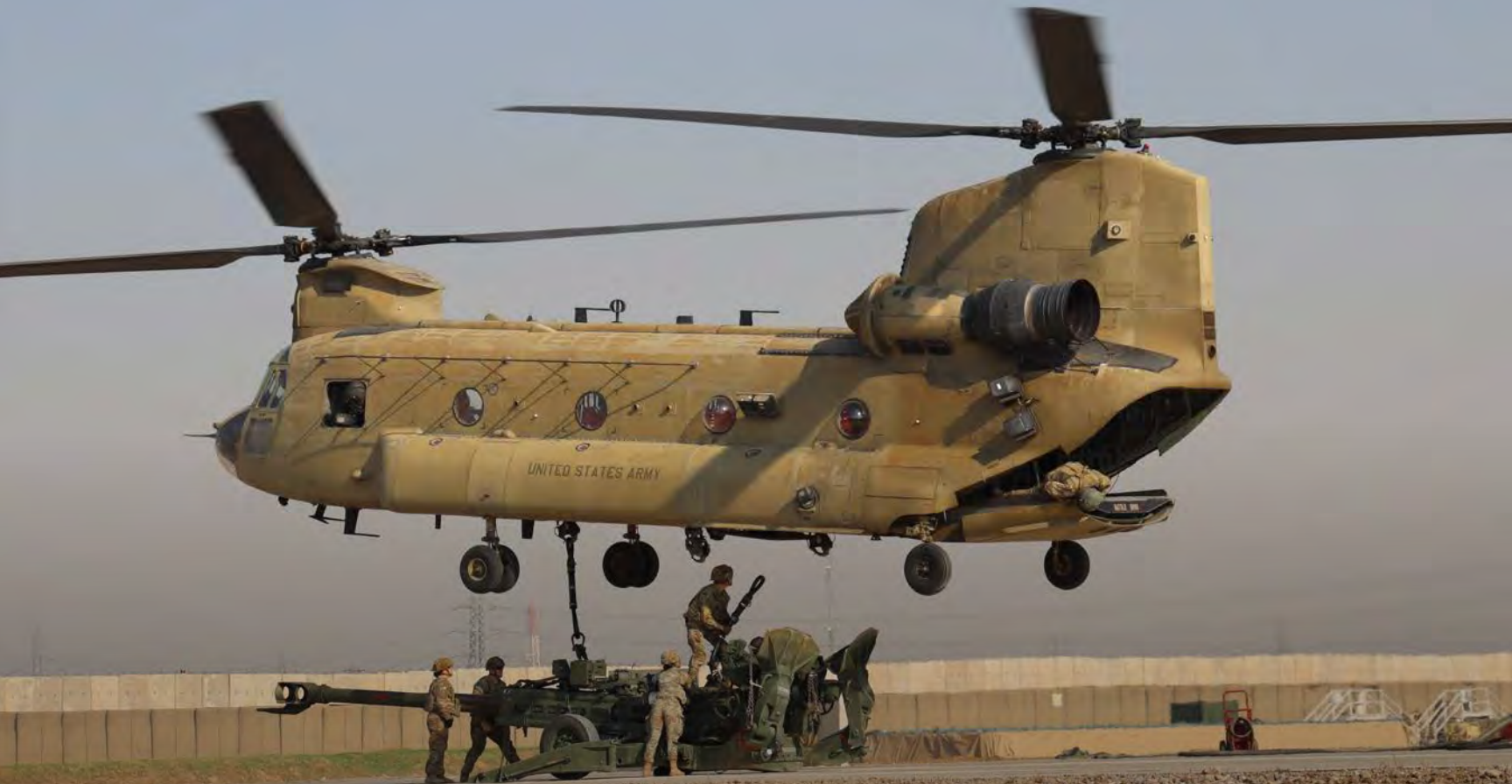
A CH-47 Chinook helicopter, operated by Soldiers with Company, 3-238th General Support Aviation Battalion, 28th Expeditionary Combat Aviation Brigade sling loads an M777 Howitzer during an exercise with Soldiers with the 2-319th Field Artillery Regiment.
